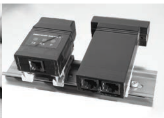
Figure 9. Typical Installation of DIN Rail Mounted Devices
