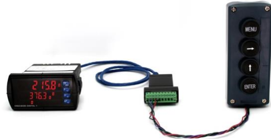
Figure 29. Meter to Control Station Connection
