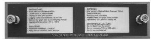
Use new, premium quality Alkaline D-Cell batteries only (Energizer E95 or Duracell/Procell MN1300).
