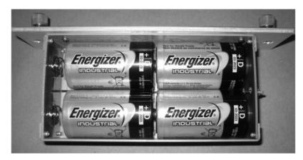
Replace the battery box and tighten thumbscrews.
