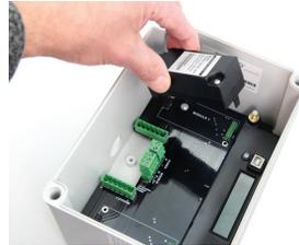
Plug the module pins into an available module port on the base station's main board as shown in the photo on the left.
