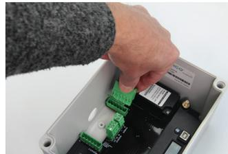
Install the connector plug into the terminal on the base station's main board. It is recommended that the wires be inserted into the plug and screws tightened prior to installing the plug into the terminal.
