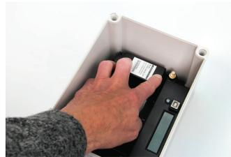
Press the module firmly onto the electronics board to make sure it is in place and secure.
