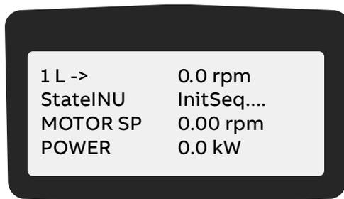
After another few seconds, the display changes to the actual signals display. The status line of the display alternates between DCGndNopen and NotReadyOn.
