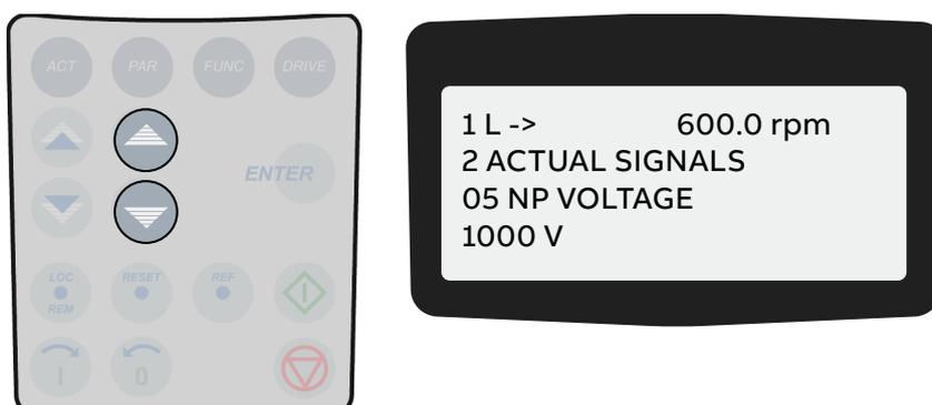
6. To confirm the selection and to return to the actual signals display, press the ENTER key.
