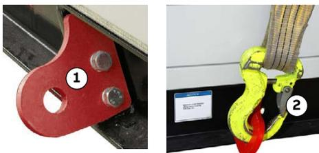
Figure 4-1 Lifting bracket on base frame of a drive and safety hook secured to lifting bracket
