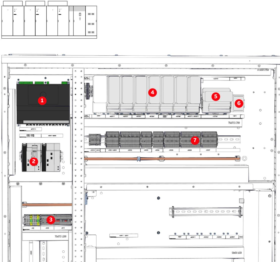
Figure 3-15 COU customer interface section
