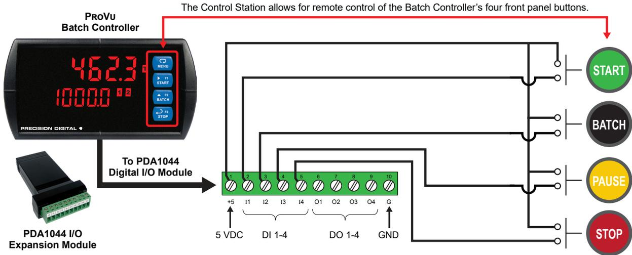
Use the PDA2364-SBPS to remotely operate the ProVu Batch Controller
