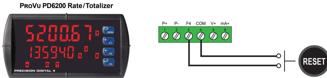
Use the PDA2361-R to reset the total on a Precision Digital rate / totalizer. The reset terminals connect to the F4 terminal on the Precision Digital meter.
