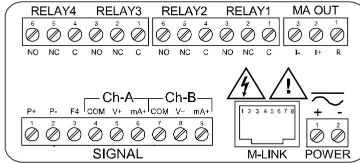
**Figure 3. Connector Labeling for Fully Loaded PD6060**
