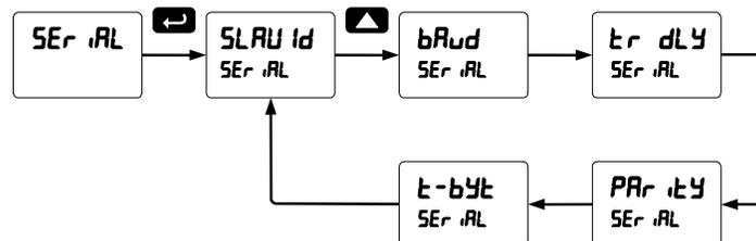
When using more than one meter in a multi-drop mode, each meter must be provided with its own unique address. The meter address (Slave ID) may be programmed between 1 and 247. The transmit delay may be set between 0 and 199 ms. The parity can be set to even, odd, or none with 1 or 2 stop bits.
