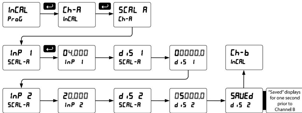
**Scaling the Meter for Channel B (SCAL-b)**
