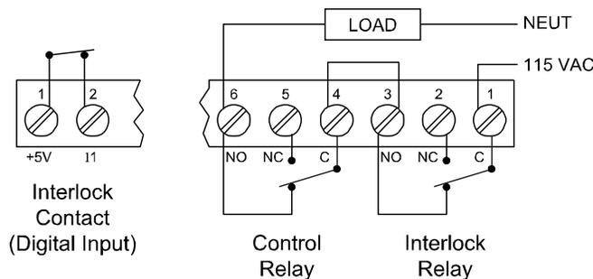
Figure 17. Interlock Connections
