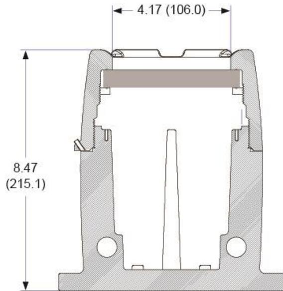
**Figure 23: Enclosure Dimensions – Side Cross Section View**
