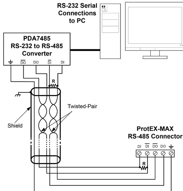
**Figure 10: RS-485 Wiring**
