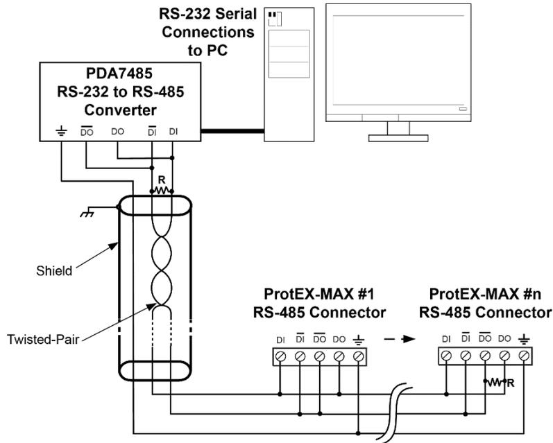
Figure 13: RS-485 Two-Wire Multi-Drop Wiring
