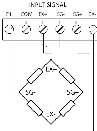
**Figure 6. Strain Gauge Powered by Internal Supply**
