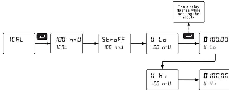
The graphic above shows the calibration of the 100 mV input range. The other input ranges are calibrated in a similar way.
