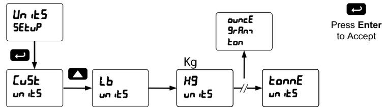
*Note: PV1 and PV2 may use different standard units as starting points, however the user must select the unit and complete scaling for both PV1 and PV2 individually. For example, set PV1 equal to "Lbs" and complete the scaling for PV1 only. PV1 is now reading in Lbs. Then, change the units for PV2 to be "Kg" and complete the scaling for PV2. PV2 will read in kilograms and PV1 will reflect the conversion from Lbs to Kgs.*
