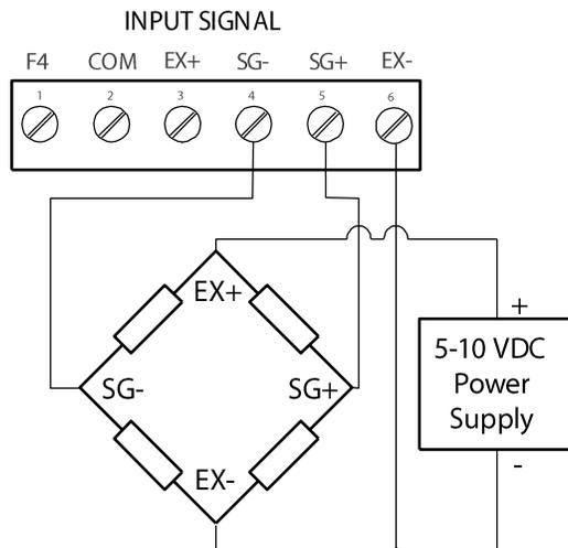
**Figure 7. Strain Gauge Powered by External Supply**
