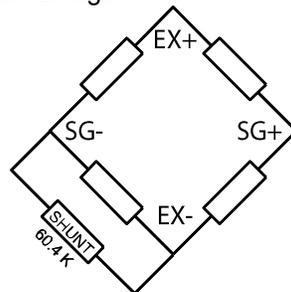
**Figure 9. Shunt Resistor**
