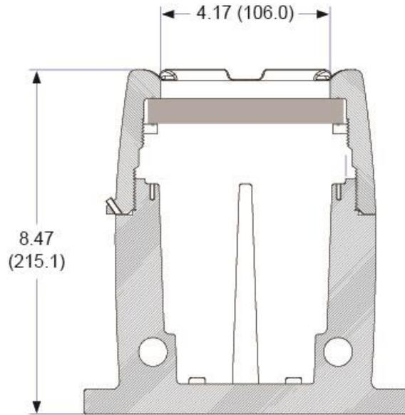
**Figure 25: Enclosure Dimensions – Side Cross Section View**
