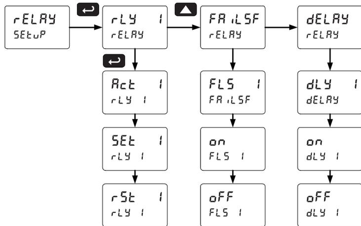
Note: The setup of relays 2-8 follows the same pattern shown here for relay 1.
