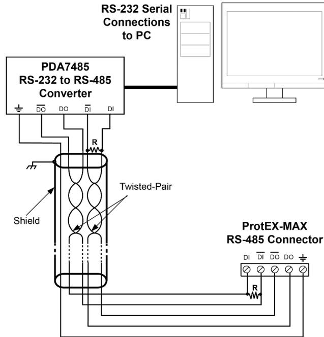
Figure 12: RS-485 Wiring
