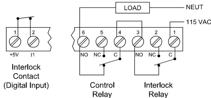
Figure 19. Interlock Connections
