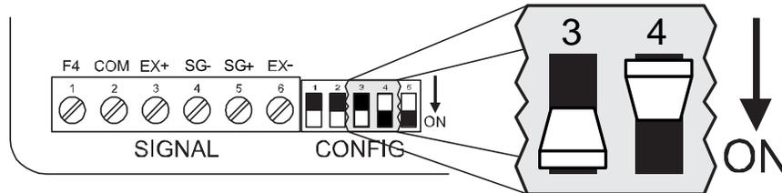
**Figure 5. Strain Gauge Configuration Switch**
