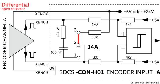
Jumper settings for differential (open collector) encoders connected to a SDCS-CON-H01
