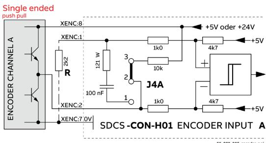
**Jumper settings for single-ended (push pull) encoders connected to a SDCS-CON-H01**
