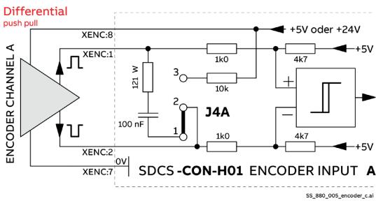
Jumper settings for differential (push pull) encoders connected to a SDCS-CON-H01
