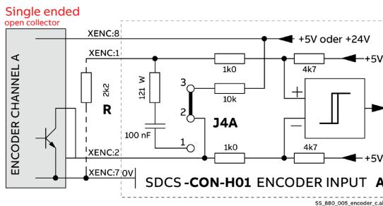
**Jumper settings for single-ended (open collector) encoders connected to a SDCS-CON-H01**
