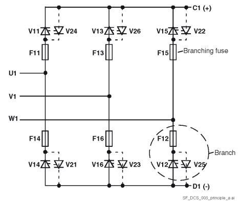
**Branch fuses installed inside converters size H7 (adapted fusing)**
