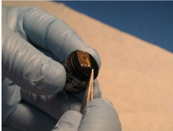
Figure 30 Spacer installation
