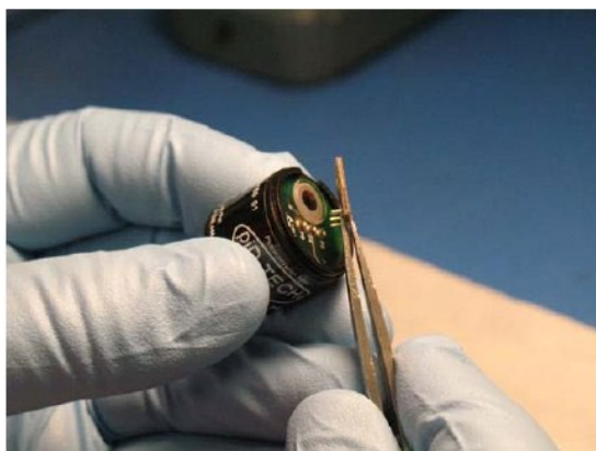
Figure 29 Cell Assembly installation
