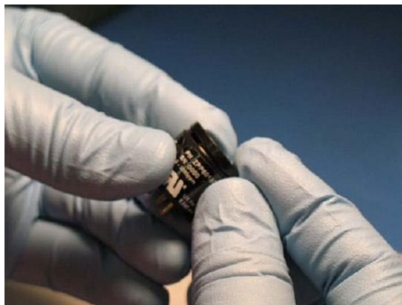
Figure 32 Replacing the Cap
