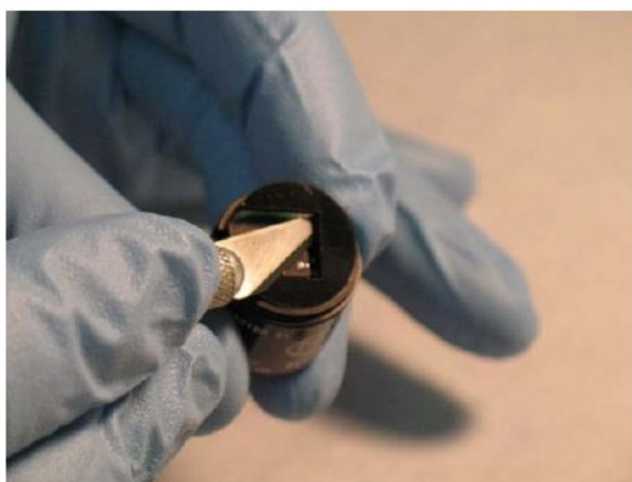
Figure 22 Removal of Spacer
