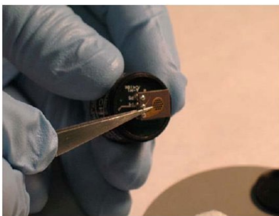
Figure 23 Removal of Cell Assembly
