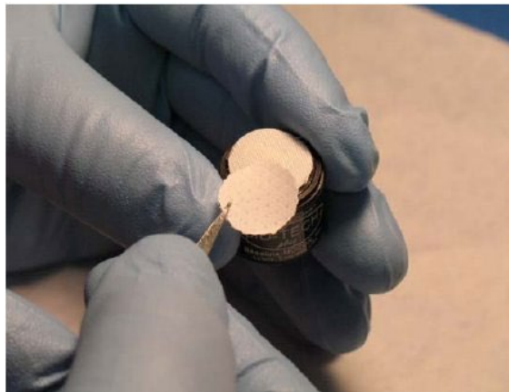
Figure 31 Installing Filter Media
