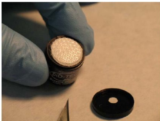
Figure 21 Removal of Filter Media
