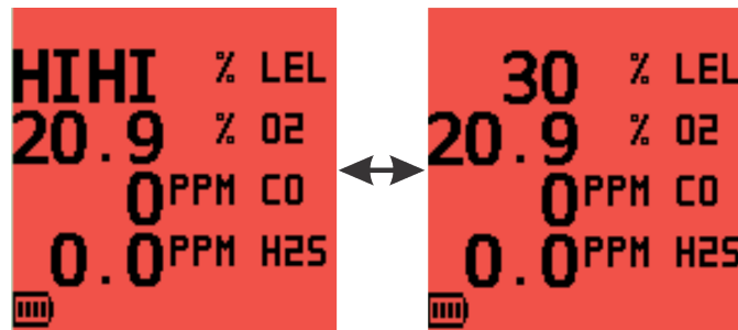
Figure 26: LEL HIHI Alarm
