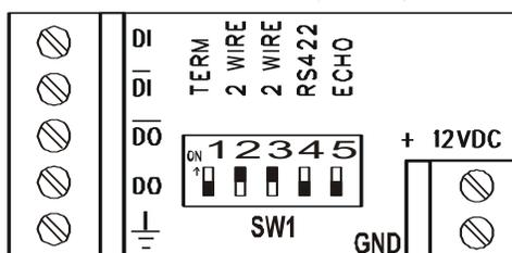
**Figure 13. PDA7485 Terminal Connectors and DIP Switch**
