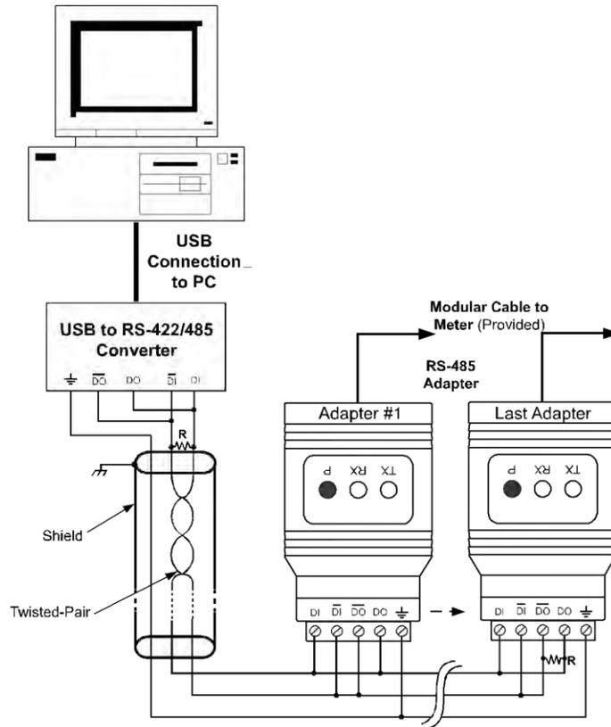
R = 120 Ohm termination resistor, typical
