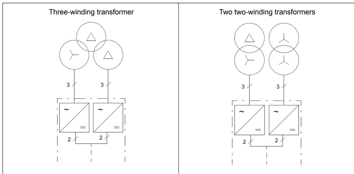
*Two parallel-connected supply units*
