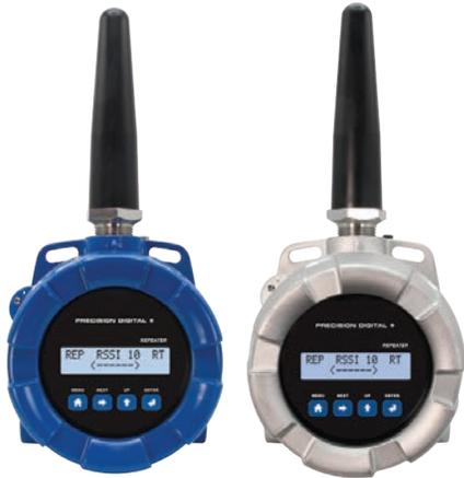
PDWR wireless signal repeaters are used to retransmit wireless signals when connectivity is an issue. They are simple to install as they only require power and a network ID. Any PDW units in range of the repeater with the same network ID will retransmit through it, thus increasing signal strength. Use repeaters to broadcast over very long distances or around permanent obstacles.
