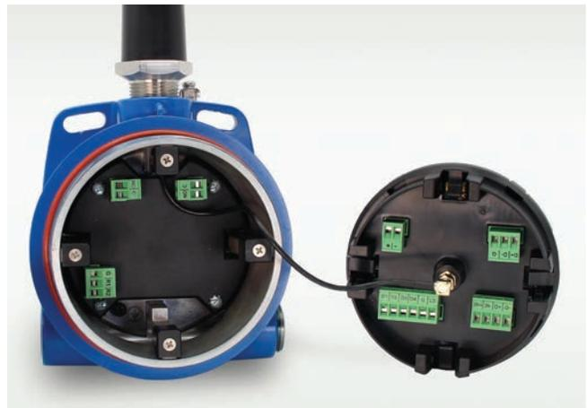
Display Module Connected to Antenna
