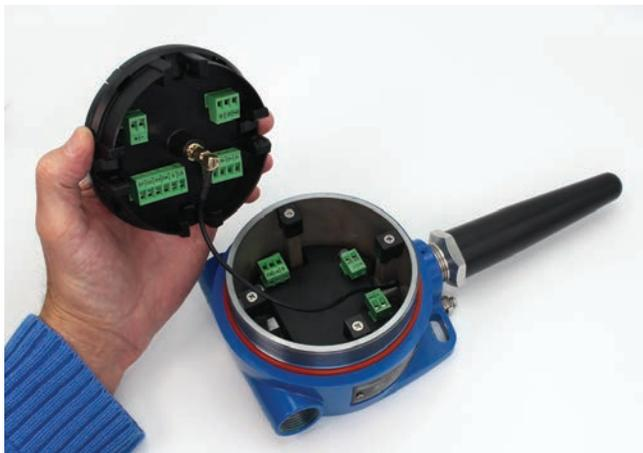
Relays Option Module Mounted on the Bottom of Enclosure
