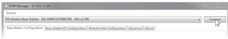
*PDW Manager* will display the following screen once data has been read from the base station. Use the tabs at the top to navigate between settings screens.
