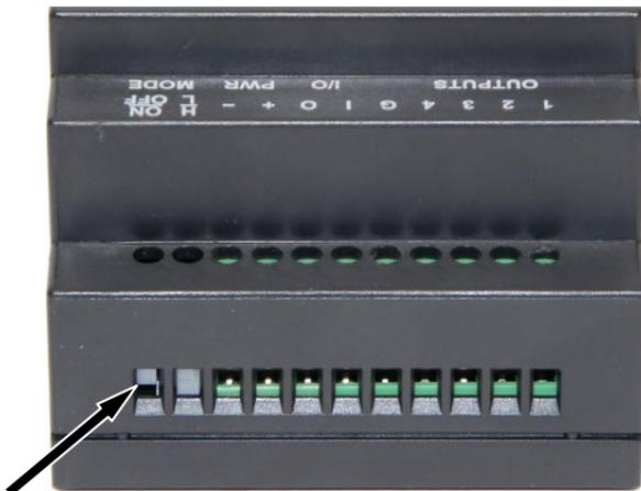
**Figure 6. Normal Mode ON/OFF (Cascade Mode) Switch**
