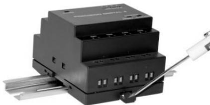
6. While pulling down on the mounting tab, rotate the bottom of the converter enclosure up until the top of the converter is freed from the DIN rail
