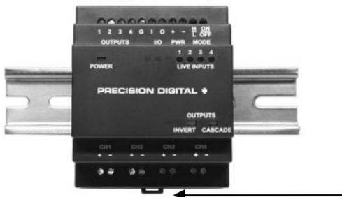
5. Insert a small slotted screwdriver or similar tool into the mounting tab, and gently pull down on it.
